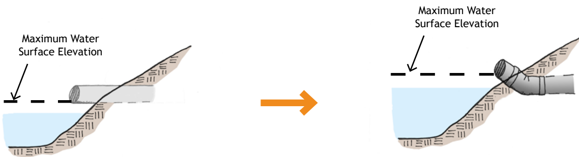
Raising the outlet pipe invert elevation.
